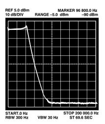
Figure 19. High Frequency Response for 9-Pole Chebychev Filter
