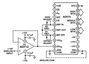
Figure 11. AD712 as ADC Unity Gain Buffer
