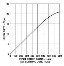
TPC 18. Slew Rate vs. Input Error Signal
