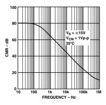
TPC 13. Common Mode Rejection vs. Frequency
