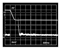
Figure 5b. Settling Characteristics 0 V to –10 V Step Upper Trace: Output of AD712 Under Test (5 V/Div) Lower Trace: Amplified Error Voltage (0.01%/Div)
