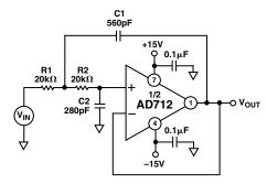
Figure 15. Second Order Low-Pass Filter
