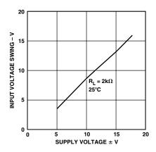
TPC 1. Input Voltage Swing vs. Supply Voltage
