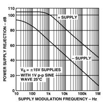
TPC 12. Power Supply Rejection vs. Frequency
