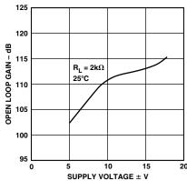
TPC 11. Open-Loop Gain vs. Supply Voltage
