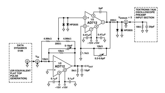
Figure 6. Settling Time Test Circuit
