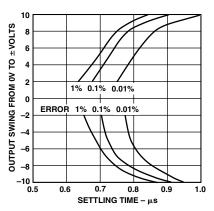
TPC 15. Output Swing and Error vs. Settling Time
