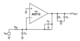
Figure 3b. Simplified Model of the AD712 Used as an Inverter
