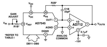
Figure 8. Unipolar Binary Operation
