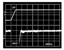
Figure 5a. Settling Characteristics 0 V to +10 V Step Upper Trace: Output of AD712 Under Test (5 V/Div) Lower Trace: Amplified Error Voltage (0.01%/Div)
