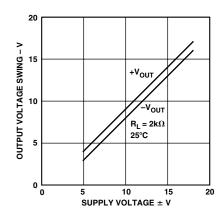
TPC 2. Output Voltage Swing vs. Supply Voltage
