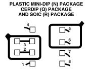
Figure 7. Board Layout for Guarding Inputs
