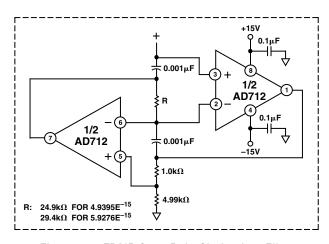
Figure 18. FDNR for 9-Pole Chebychev Filter
