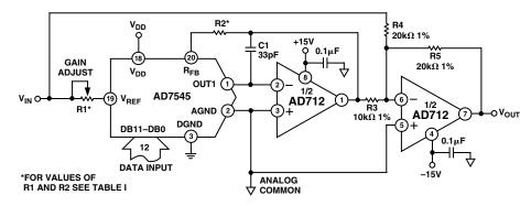
Figure 9. Bipolar Operation
