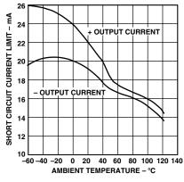
TPC 8. Short Circuit Current Limit vs. Temperature
